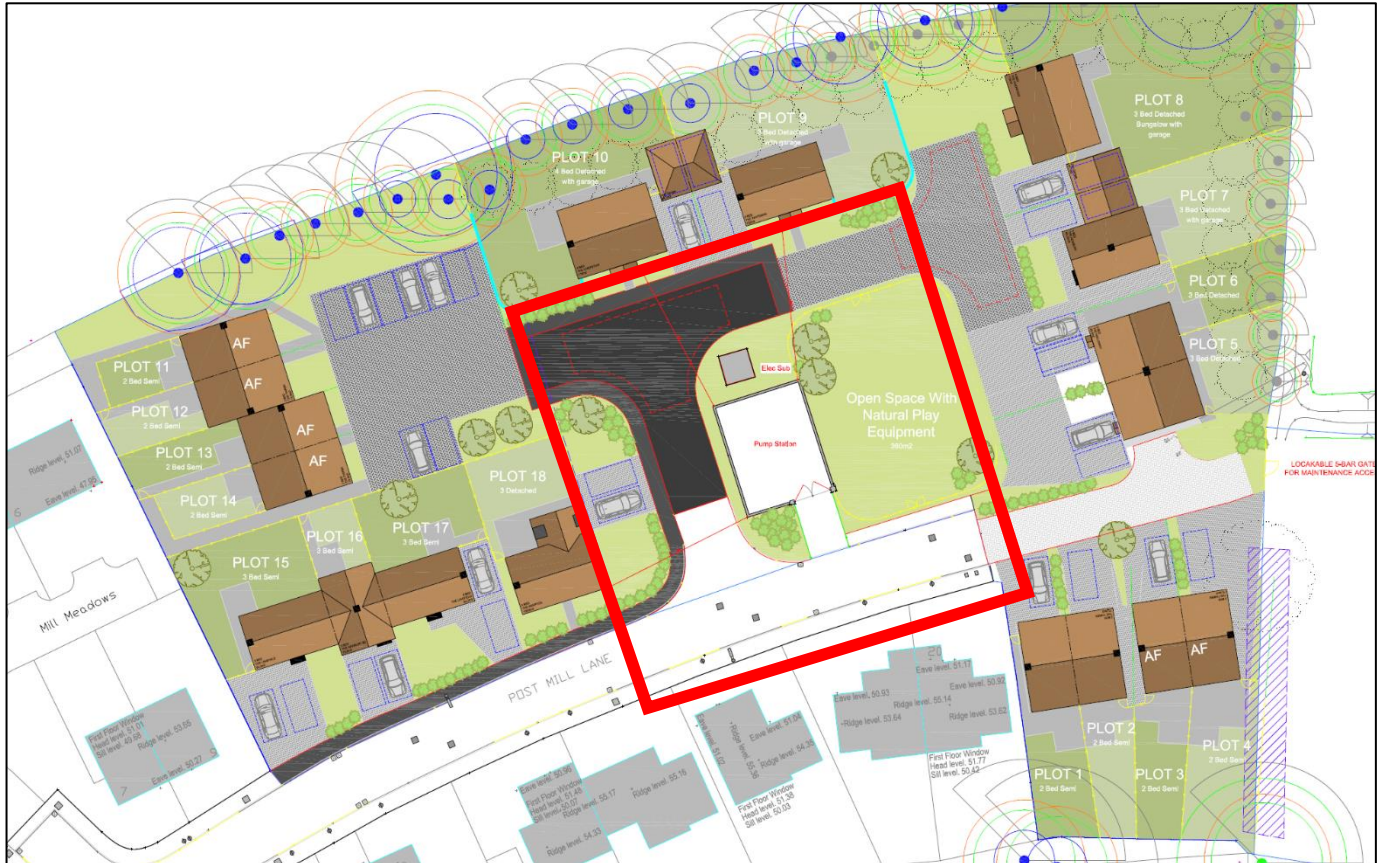
figure19: Amended layout with dwellings set back beyond a 15m pumping station
